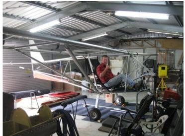
Mal has the wings on, all the control surfaces fitted and operational, and the throttle lever fitted as well. He has also installed the 90 litre fuselage fuel tank and fuel lines. Additionally, he has installed the elevator trim control and has the flaps working. As can be seen from the photo at right, he has the panel installed and is mocking up the instruments too. He told me just this week that he is covering the rear fuselage.
