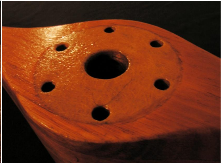
After epoxy repair
