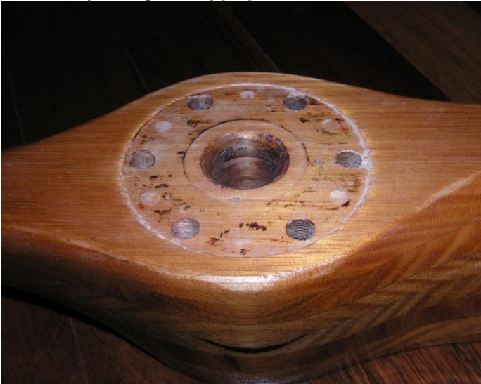
Crushed (over-tightened) propeller
