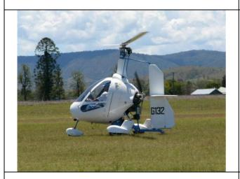
Slick looking gyro seen at Watts. This one is a two seater with a tall tail and a prerotator to spin up the main rotor to help the take off run. It is an impressive well built machine powered by a Rotax 912. The gyros are often seen at Watts Bridge with a small but very dedicated group who bring them out for some local flying and testing.
