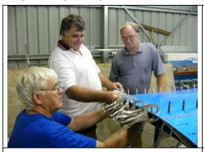
Danny and crew are busy working on the wing tip of the Zenair CH 701 they are building. One wing is nearly finished with one to go. The fuselage structure is nearly completed with the horizontal stabilizer, elevator and rudder fitted with the controls being tried. Work continues on the wing tanks and flaperon assembly. Progress is continuing at a good rate.
