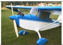
aircraft, designed by Wayne Ison, date back to the mid 1980's. The range includes the mid wing MiniMax and the high wing Himax which share a common fuselage and wing structure. For the homebuilder several choices are available such as plans only, partial component kits to full kits at reasonable costs. Engines up to 45 horse power are suitable and range from Rotax 277 to 503, Zenoah to VW 1600.
