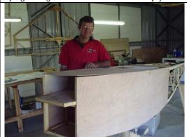
New QUA member Tony Wright is on the left with some of the components he has assembled from a kit supplied by JDT Aircraft. Tony has already constructed the wings, tail surfaces and is now working on the fuselage for his Himax which will be powered by a Rotax 477 engine. Performance expected is a cruise speed of 60 knots, climb rate of 900 feet per minute and a takeoff roll of 35 metres. Tony has also prepared an excellent web site with many photographs of the construction stages.
