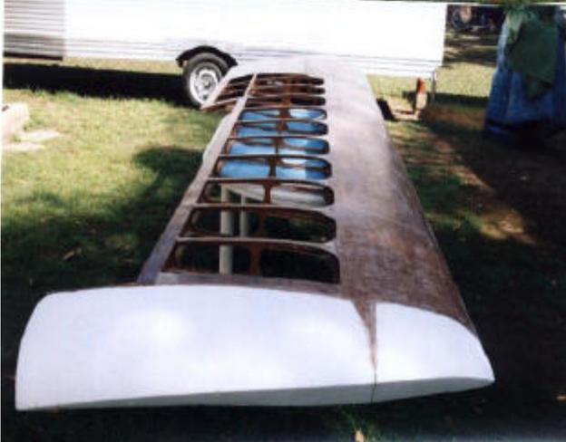
On reading different specifications on wooden aircraft I discovered that to buy spruce in Australia was quite expensive. Hoop pine was then used to make the main structural parts, making sure that there were at least 12 growth rings per inch (minimum) quite often more is satisfactory. The marine ply that was used for covering is called Gibboon as it is less weight than ordinary marine ply.
