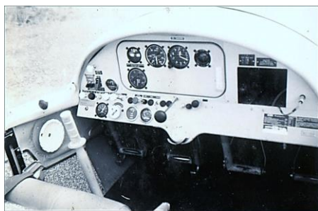
MS880B Rallye, ZK-CBT's cockpit (VHF radio missing). The big white wheel on the left is the elevator trim.
