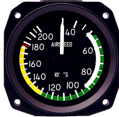
The standard type ASI fitted to most light aircraft.
