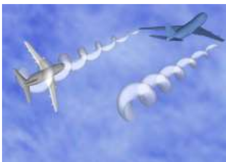
Aeroplanes leave two horizontal, inward revolving corkscrews in the air, making a net downdraft behind the aircraft
