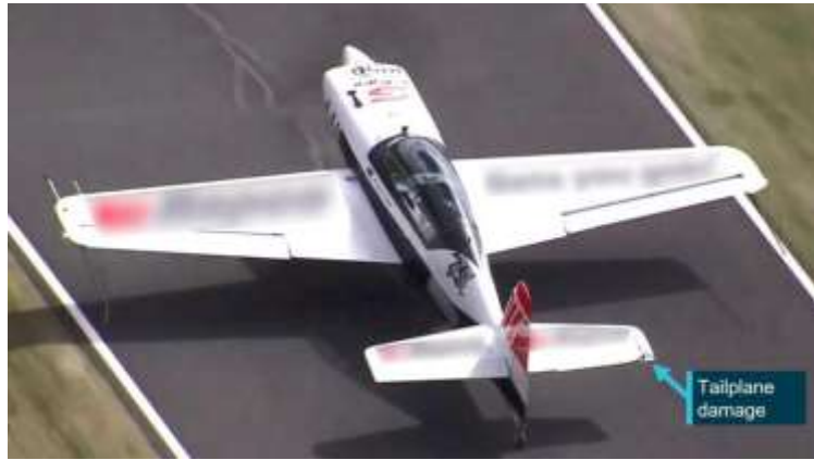
The Extra EA 300-LT aircraft sustained tail damage after landing on the race track on Mt Panorama in 2024. (Supplied: Australian Transport Safety Bureau)
