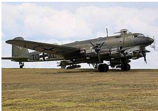
FW 200 Condor, fitted with torpedo and gun turrets.
