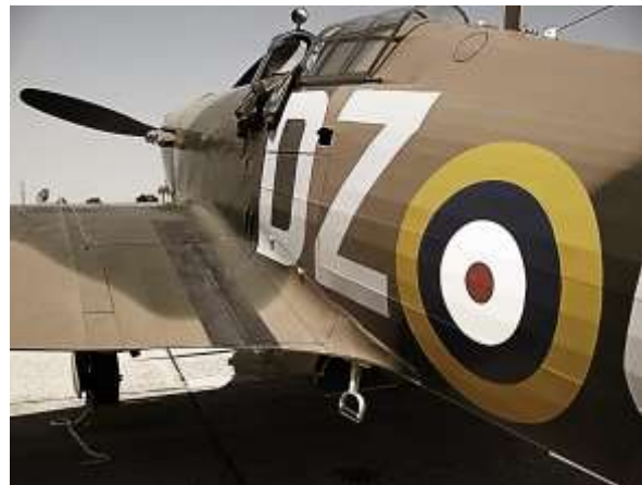
The fabric covered fuselage and pilot's foot step for entering the cockpit.
