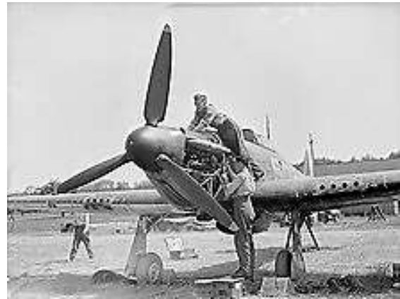
Mechanics servicing the engine of a Hurricane I of 501 Squadron, at No. 1 Repair Centre, Reims, Champagne, in France, in 1940. Note the four gun-ports in the leading edge of each wing
