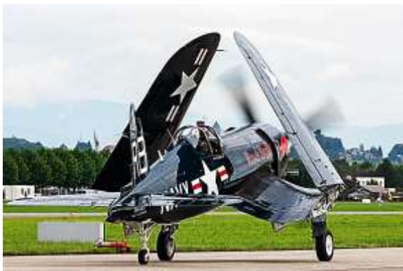
Korean War F4U, taxiing with wings folded. Note the poor pilot visibility ahead requiring "S" turns to see ahead.
