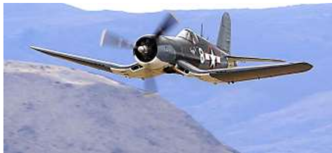
The F4U Corsair, note the two radiators built into its gull wings.
