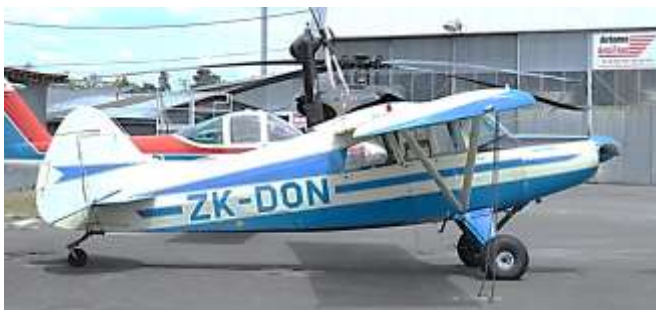
DON, with its classic Pacer tail. In later models, its profile was changed and enlarged by some 30%, along with the tailplane and elevator.
