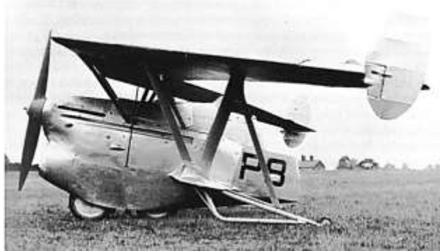
The Pterodactyl, Mk.V, fighter in 1934. Pilot up front, gunner in the back.
