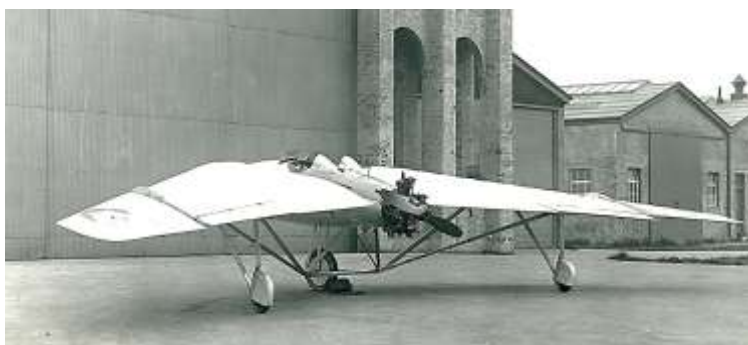
The Pterodactyl Mk.IB with the Genet engine fitted. Note that the apparent ailerons fitted inboard of the controllers are the dive brakes fitted to this Mk and provide no roll control.
