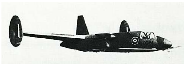
The slim lines of the 5/8ths scale M.39B with two DH Gypsy Major 140 hp engines.
