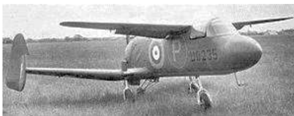
The unique Miles M.35 Libellula. Notice the “down” elevators on the front wing that would have provided a nose-ditch up in this aircraft.
