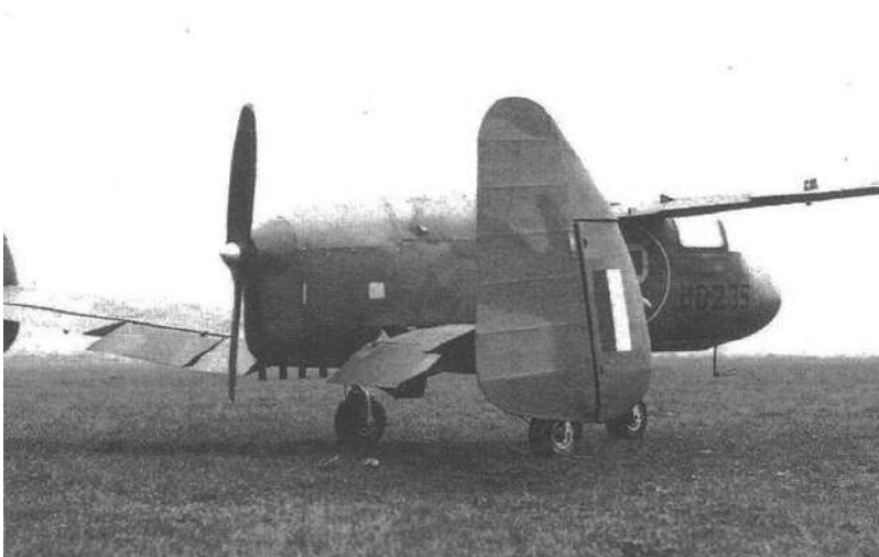
Miles M.35 Libellula, after its first flight on 1 May 1942. Note the flaps lowered on the rear wings.
