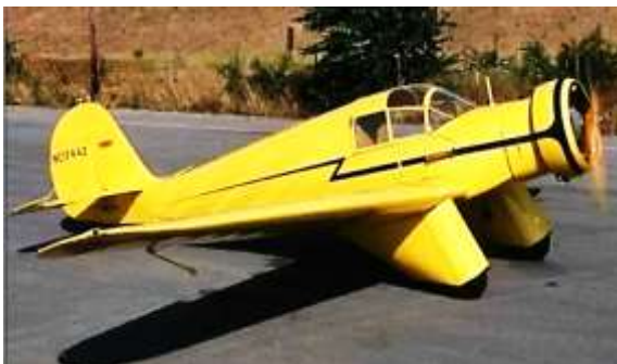
Aeronca L series. Note the clean lines, no struts, wheel and undercarriage pants, and the townsend ring around the cylinders on the engine, all drag reducing elements.
