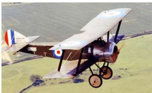
Original Sopwith Pup N5195 is now displayed at the Museum of Army Flying. The cowl, with a lower cutaway vent, indicates this aircraft powered by an 80 hp Le Rhone engine.
