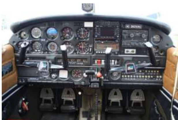
A PA28 Warrior panel. The circuit breakers are on the right, below the control yoke.
