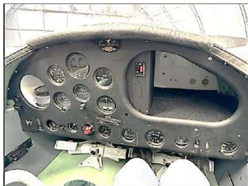
The AKE Panel. On the far left is the compass. Image courtesy of Michael Bach.
