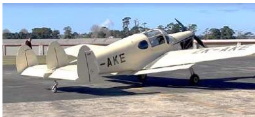
Miles M.38 Messenger IIA, with its lower engine cowl removed, about to commence brake trials. Image courtesy of Michael Bach.
