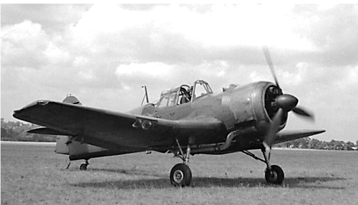
An M.19 Master II with a Bristol Mercury engine. Note the glider tow apparatus behind the tailwheel.
