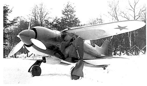
The IS-2. Note the recess in the top wing underside to house the retracted lower wing.
