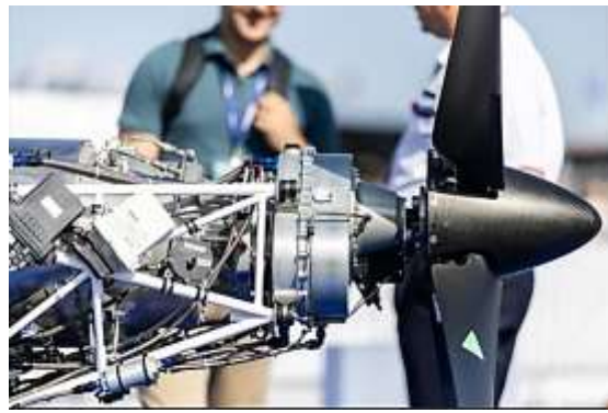
The TP-R90 turbine engine designed for light GA aircraft
