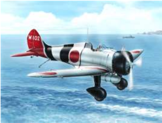
Mitsubishi A5M (Type 96) Claude fighter with jettisonable belly tank carrier arrester hook.
