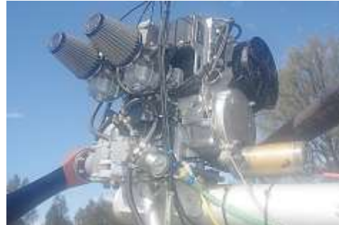
New Engine Rotax 503 Dual Ignition has only 10
