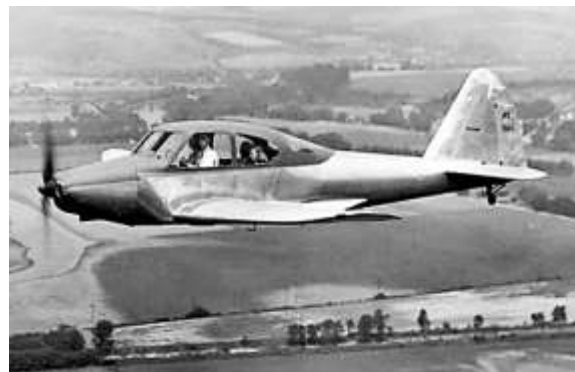
The 1947 second prototype Piper PA-6 Sky Sedan with a stressed skin construction.
