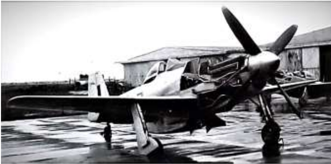
The nearly completed airframe fitted with the R-R Griffon 61 V12.
