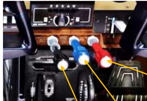
Cessna182, vernier type knob engine controls. Standard colour code – BLACK throttle, BLUE pitch (RPM), and RED for Mixture
