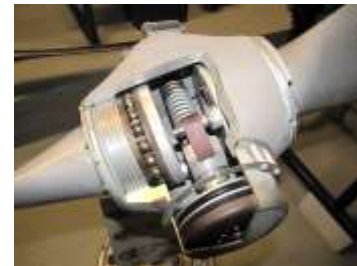
Cutaway showing the complexity of a CSU propeller hub.
