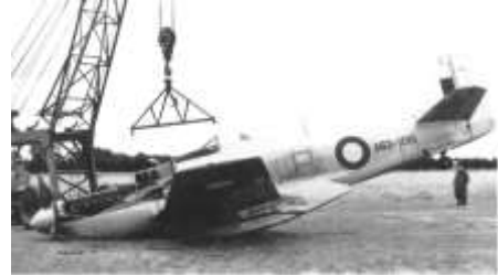
Wheels-up - post hydraulic failure.
