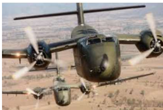
The iconic high gull wing design of the Caribou made it very distinctive in flight, reduced the length required for the undercarriage legs, and aided lateral stability.
