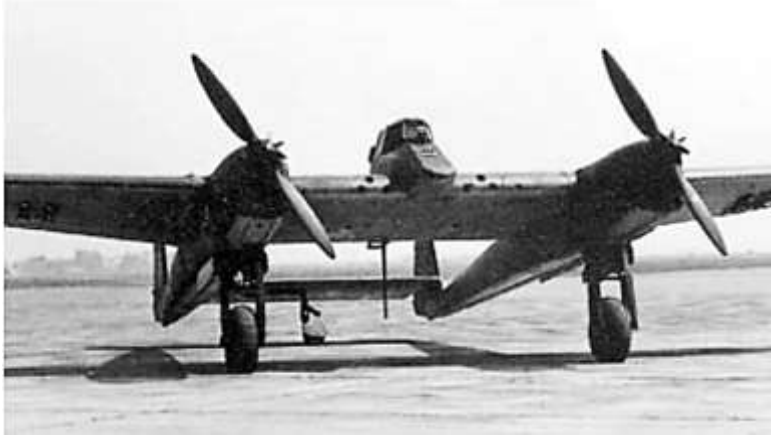
The cramped Focke-Wulf Fw 189C cockpit was home to a crew of two, seated back-to-back - the pilot facing forward and the gunner, aft.
