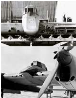
A major modification in the Fw-189C was the replacement of the large glazed, hi-viz cockpit with a heavily armoured central nacelle for protection from ground fire.
