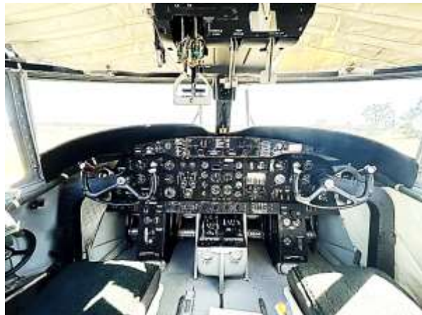
The Caribou flight deck – note the throttles and other controls in the roof.
