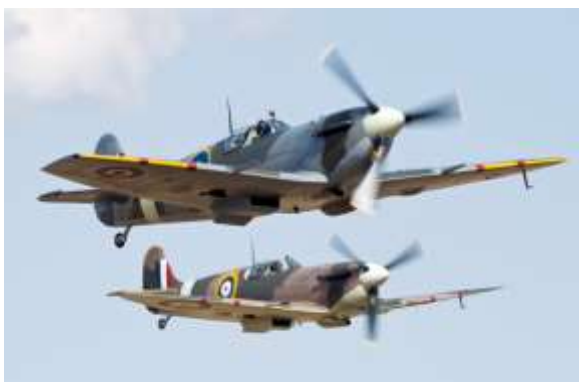
Spitfires in formation. These are different Mk's, note the clipped wing-tips on the nearer aircraft.
