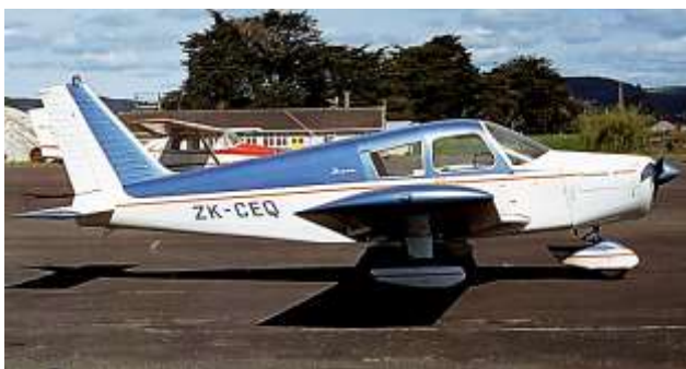
At Ardmore, New Zealand, ZK-CEQ, no 52 off the first production line of the PA-28-140 in 1964. Note the aerofoil shape at the wing tip. Serial number is 28-20052
