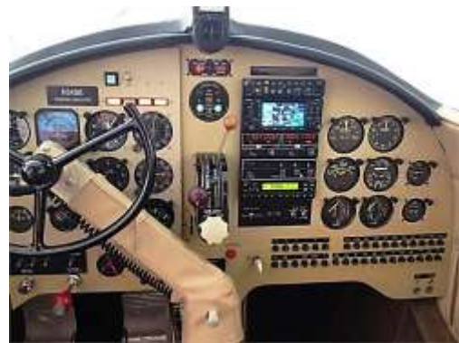
A typical Spartan panel with the cross-over yoke control.
