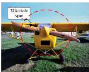
Most thrust is produced at about 75% out from the propeller boss.
