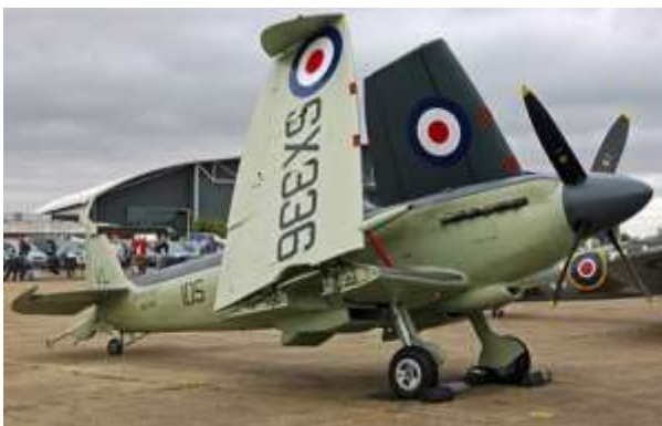
Seafire, Griffin engine, and folding wings, looking for an aircraft carrier.
