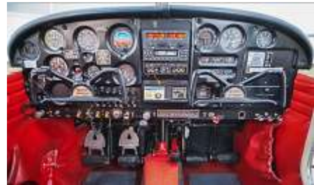
A 1964 PA-28-140 panel with a black push/pull throttle and red mixture control.
