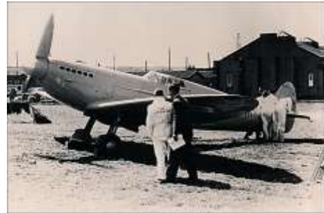
K5054 – The Spitfire prototype. Note the large chord length and course fixed-pitch on its wooden propeller.
