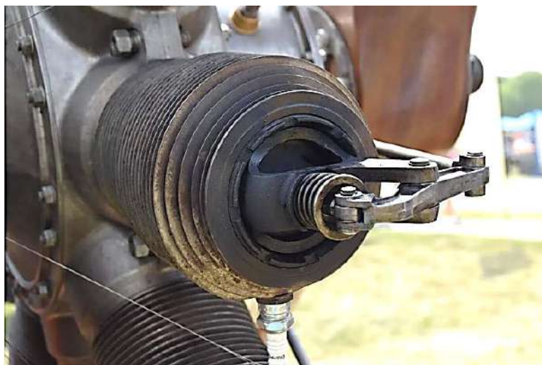
The pushrod-activated exhaust valve on top of the cylinder
