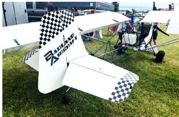
F-1 (named after the tornado scale) ultralight with folding wings.
