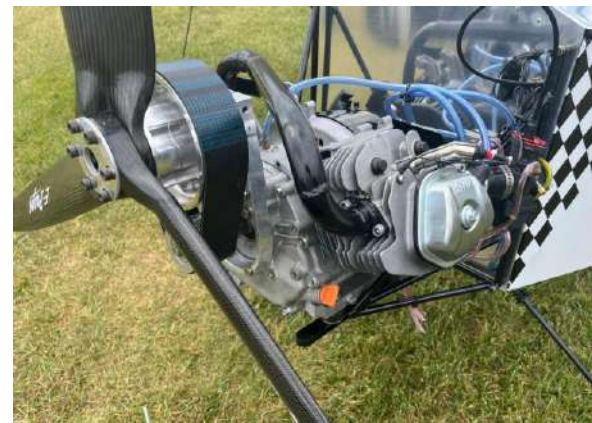
Thump Air single cylinder four stroke engine, with Badland re-drive, based on a Honda industrial engine.
