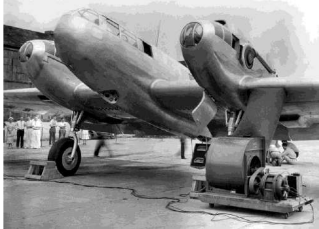
Electric fans, ducted into the Airacuda's leading-edge intakes, provided much-needed cooling air during engine runs on the ground. [Credit: U.S. Army Air Forces]
