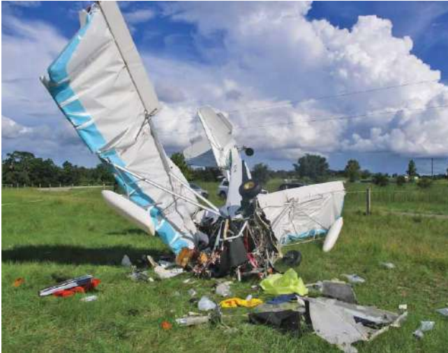
The owner of this Aventura had been in the process of modifying the carburetion. NTSB investigators found the top spark plug to be black and sooty, consistent with the Rotax 912 engine running
