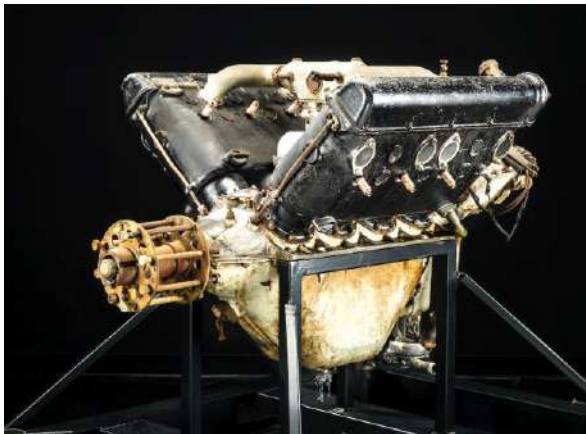
A Wright-Martin Model E, licensed version of the Hispano-Suiza SOHC V-8 aircraft engine, in the collection of the Smithsonian Institution, National Air and Space Museum. (NASM 2014-04437)
