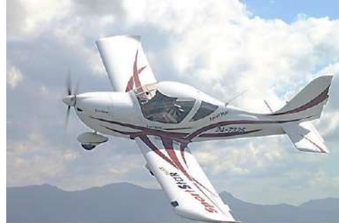
The whole time the propeller is turning clockwise, the airframe's trying to turn anticlockwise.
