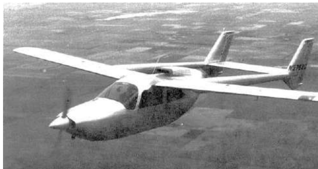
One of the few publicly available photos of the Cessna 327 prior to its time with NASA. In this view, the compact fuselage, sleek windscreen, and lack of wing struts are evident. [Credit: Cessna]
