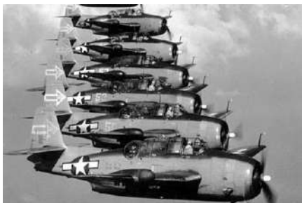
Seven Grumman TBM-3D Avenger bombers of night torpedo squadron VT(N)-90 flying in formation in January 1945. The squadron was part of Night Air Group 90 on the carrier USS Enterprise. Note the radar pods in right-side wings, and the distinctive tail insignia. [Photo: William T. Barr/U.S. Navy]
