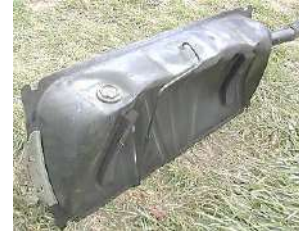
Fuel tank collapse caused by a blocked vent
