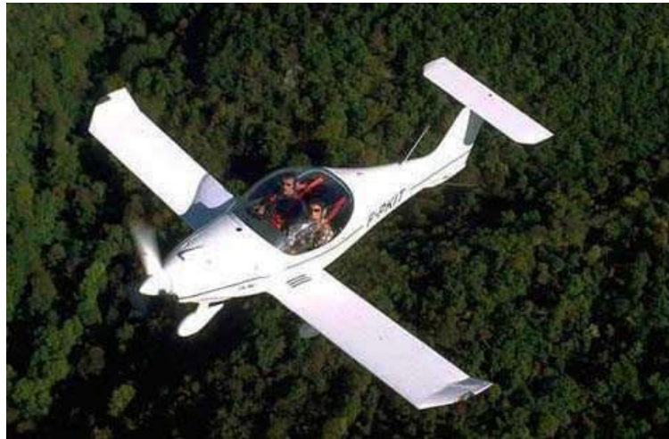
The Dyn'Aéro MCR01 is a two-seat, low-wing, all-composite carbon fibre light aircraft that was originally manufactured by Dyn'Aéro in France, and is now available both in kit form and ready-to-fly. It is powered by a 100 hp Rotax 912.engine.
