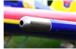
The pitot tube. When the opening does not point directly into the airflow, the tube recognizes a reduced dynamic pressure so the ASI will read a lower than correct airspeed.
