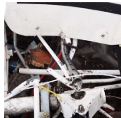
The damage to the pilot’s seat in the Escapade plane (AAIB/PA)© Provided by PA Media
