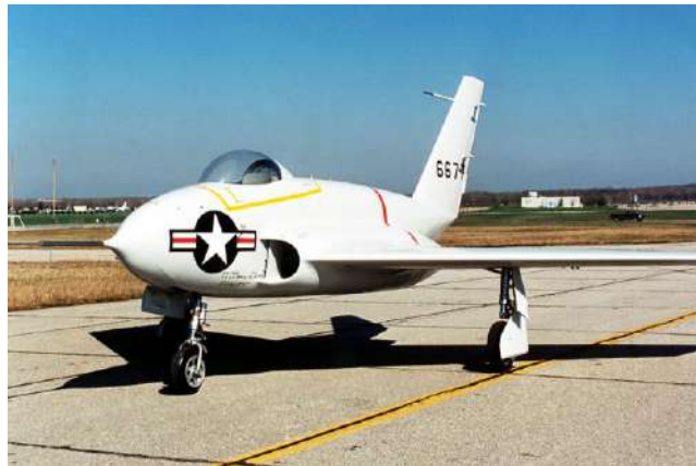
The simplicity of the X-4's semi-tailless airframe is evident in this photo. [Courtesy: U.S. Air Force]
