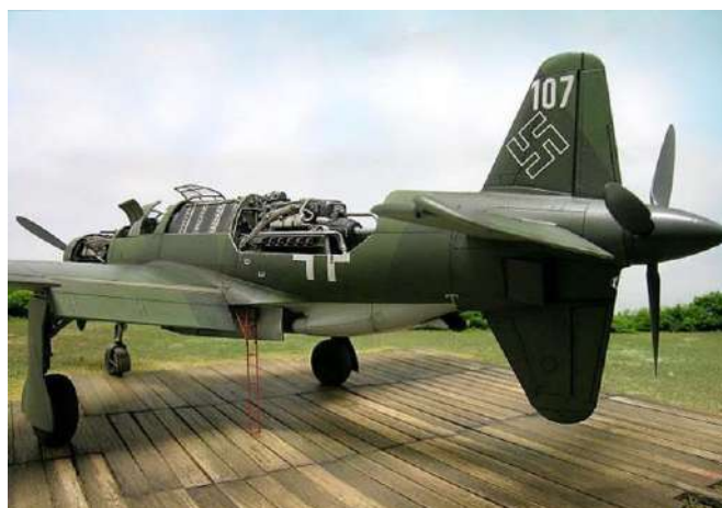
DO 335 with engine covers removed. Each engine had a capacity of 44.5 litres and weighed 910kg
