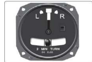
A “bat & ball” slip/skid instrument
