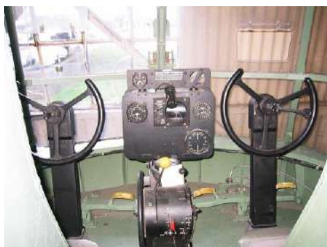
AS.51 cockpit. Even the control wheels were made from wood
