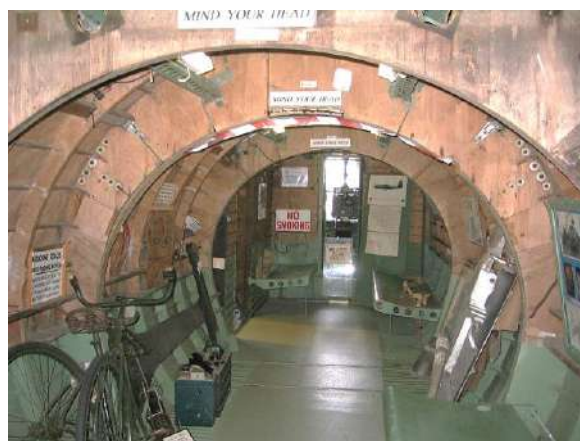
All fittings and wooden frames were exposed
