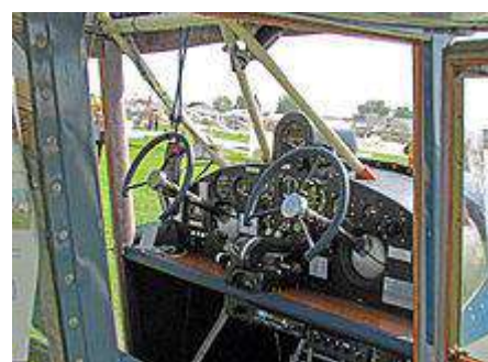
Cockpit detail showing the unusual twin "steering wheel" controls jutting out from the instrument panel.
