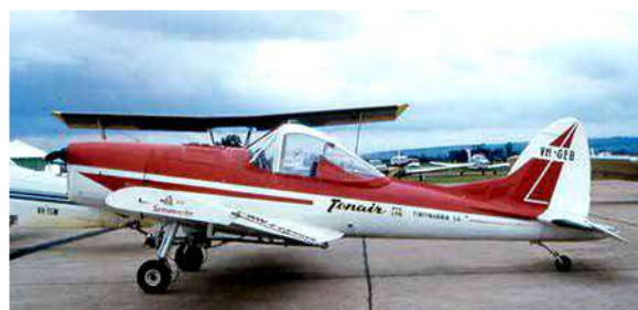
In 1965 Chippy was converted as third SA-29 Spraymaster at Bankstown, Australia, and recertificated as VH-GEB. Mods include forward part of fuselage interior and front seat removed to install a hopper, rear seat raised, and single seat bubble canopy installed. It also received a dorsal fin, Scott-style tailwheel, and attachments for spray equipment and controls (skin holes and doublers still very much in evidence today!) It still had the stock 145-hp Gipsy Major engine. It flew out of Tintinara, Southern Australia, landed in a field and was badly damaged. Once repaired, it continued to operate as a Spraymaster until 1969.
