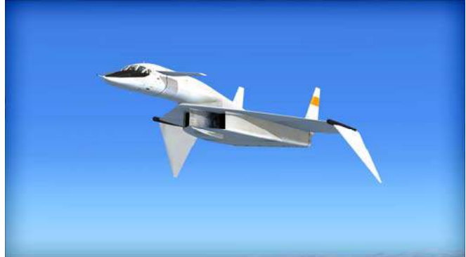
The XB-70 Valkyrie in flight. Note the in-flight, droopable wing tips that allowed the aircraft to ride on its own supersonic shock wave.
