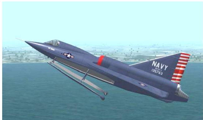
An XF2Y-1 in flight with hydro-skis extended
