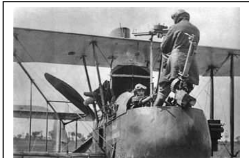
The gunner's position. Note that his cockpit depth is only ankle deep. No seatbelt, either!
