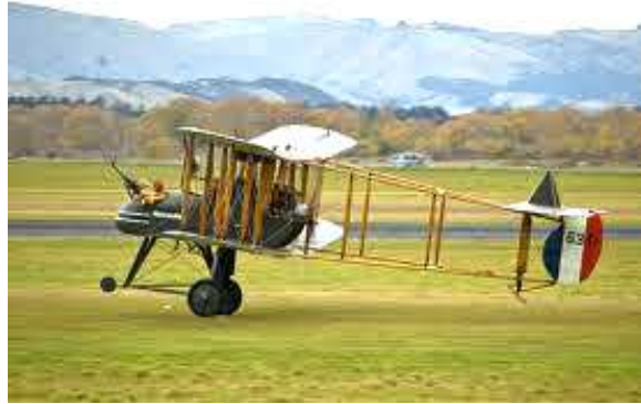
Replica F.E.2B at Hood Aerodrome, at Masterton, New Zealand. This is the only F.E.2B flying anywhere in the world and has an original Beardmore engine powering it
