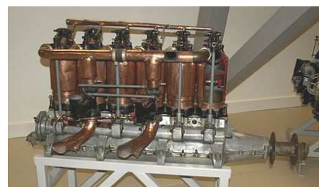
16 litre, 160 HP Beardmore engine weighing 279 kg. (Wikipedia)
