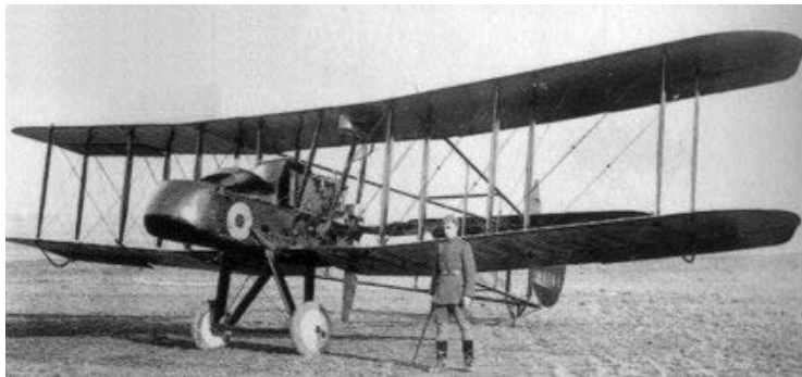
The FE.2B (Image from Wikipedia), the development of a design originating in 1910 with the F.E.2 design. This one not fitted with the two machine guns, one facing forward, the other aft, in the front cockpit.
