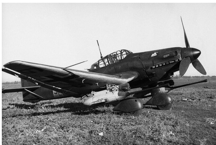
Armed with powerful 37mm Panzerknacker anti-tank cannons, the Ju-87G traded the role of dive bomber for that of a potent tank killer. (National Archives)
