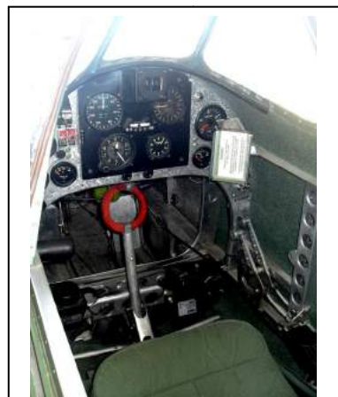
The cockpit right side showing the two undercarriage retraction levers
