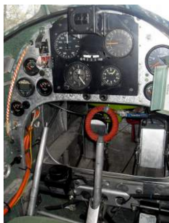
The cockpit (left side) showing stick and silver flap lever
