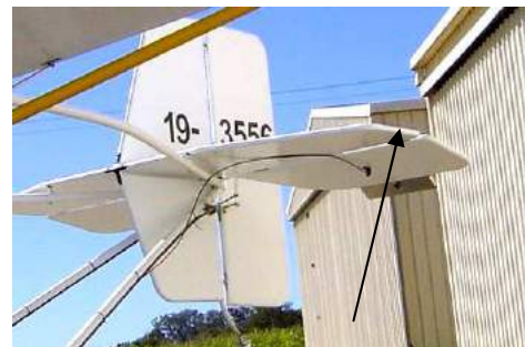
Elevator trim tab fixed to the trailing edge of the elevator of a Genesis.
