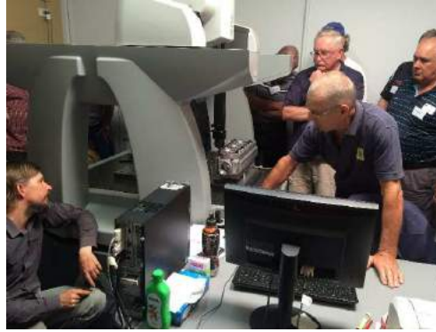
Computer operated machine with fine needle heads used to take measurements of crankcase: very much like a dentist drill
