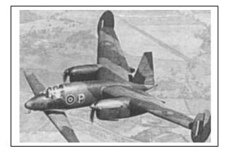
The Miles Libellula, a Second World War tandem wing experimental aircraft built by Miles Aircraft in England, designed to give the pilot the best view possible for landing on aircraft carriers. It first flew in July 1943.
