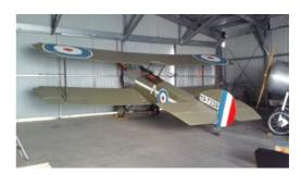
VW 2275cc geared engine and this engine has now been replaced with a Lycoming O-320 and a new prop. This was done without any changes to the weight (removal of lead ballast replaced by heavier engine). Has not flown with the Lycoming yet but flew very well with the VW engine.
