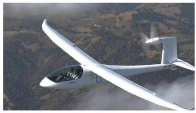
The E-Genius, a 2 seat, electric driven, powered glider
