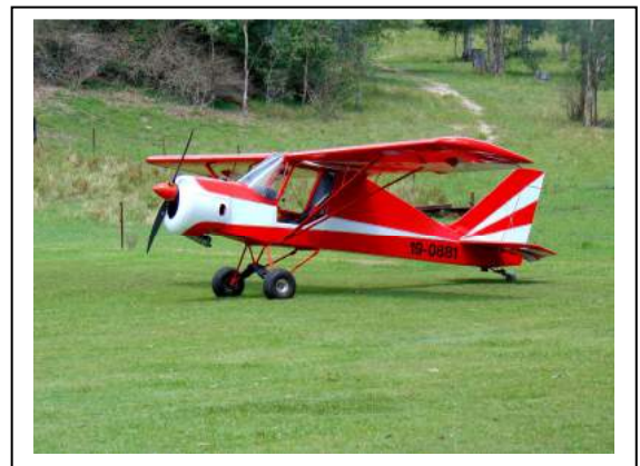
Shaun Winson's Mark 2 Superpup. With a Rotax 582 under the radial style cowl, this little aeroplane has a reputedly sparkling performance.
