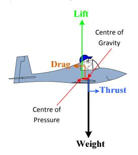
the linear distance between the Centre of Gravity and the Centre of Pressure. And herein lies the problem — as the angle of attack changes so does the location of the Centre of Pressure. With an increase in angle of attack, the Centre of Pressure moves forward along the chord. This is unstable and effectively reduces the arm and thus the strength of the lift/weight couple. This means there is less natural force to hold the nose down and the elevator must be used for attitude control.
