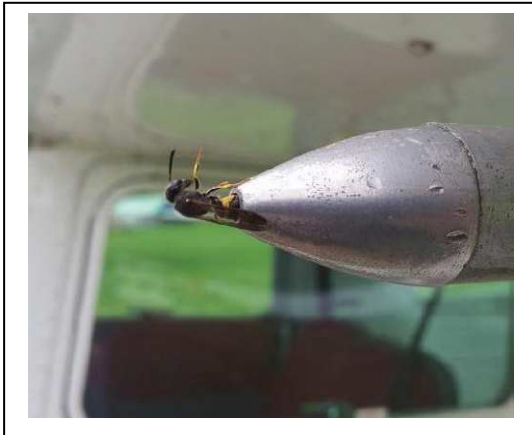
Figure 1. Mud dauber wasp emerging from an uncovered pitot tube. (Source:backcountrypilot.org)
