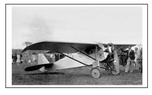
Designed and built by Geoffrey Wickner, a cousin of Edgar Percival in 1932 the Wicko Sports Cabin aircraft was the first aircraft to be completely designed and built in Queensland. Initially powered by an 80 hp Anzani radial engine, the remains of this aircraft now hang in the Queensland Museum at Caloundra.
