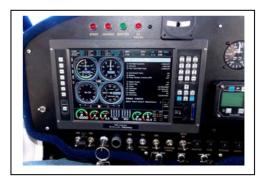
The flight and engine instruments are well laid out on the glass panel
