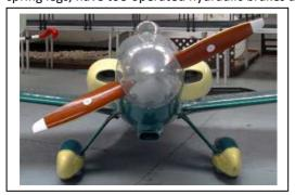
The 'Wind". Note the monstrous spinner and the tiny bubble canopy above it.
