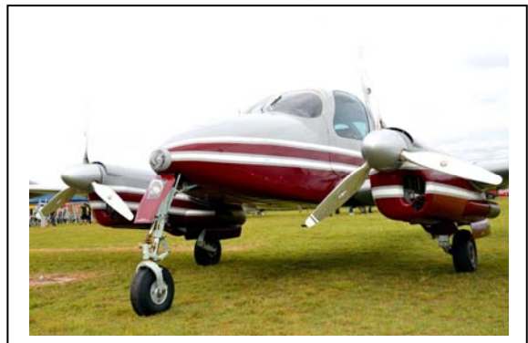
Moravia L200D, with its 210hp Avia M 337 engines
