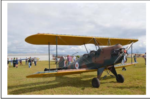
A PlatzerKiebitz homebuilt with a VW engine
