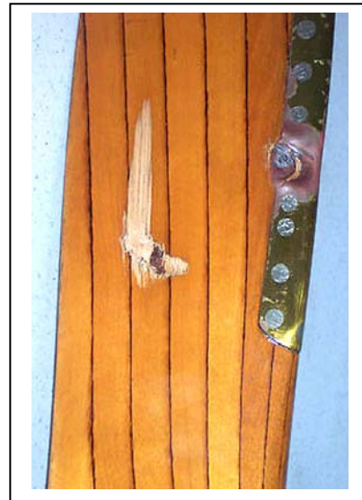
Irreparably damaged wooden propeller blade.
