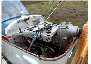
The aircraft is timber and fabric and was built by Phil Bird in Sydney about 10 years ago. It's powered by a Rotax 447 with a Sweetapple propeller and cruises between 55 and 60 knots. To say Phil did a great job is an understatement. The quality of the construction and finish really is impressive. Phil sold the Koala after six or seven years to the first of three owners in Tasmania, none of whom used it very much.
