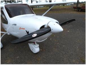
the production propellers will be fixed at that pitch. The new propeller is being used on the J170-D prototype and having taken a ride in that plane a couple of weeks after Monto I can say that the new prop is extremely smooth running.
