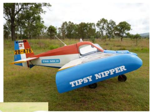
Wikipedia goes on to describe the aircraft as having a welded steel tube fuselage and rudder with a wooden and fabric covered wing, tailplane and elevator. It weighs 165 kg without an engine. Early aircraft were equipped with a 40 hp Stamo VW-engine with later types using either 40 hp Pollman-Hepu or 45 hp Stark Stamo engines.
