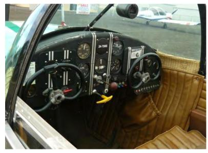
After running-up the motor, the pre-takeoff checks were simple. The Ercoupe has no flaps and an automatic mixture control, however, there are a couple of unique aspects to the pre-takeoff ritual. The sliding windows need to be raised to improve performance, and only the elevator can be checked for full and free movement – the interconnected rudder prevents the ailerons being moved unless the aeroplane is rolling or flying.
